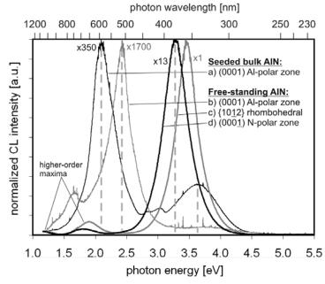
Fig. 2: Normalized CL spectra of different zones in bulk AlN.
